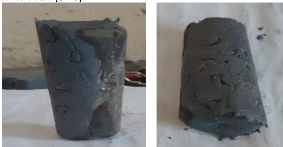
Picture 2. Samples cast in an electric arc furnace from a gray cast iron alloy in a sand-clay mold for research.
