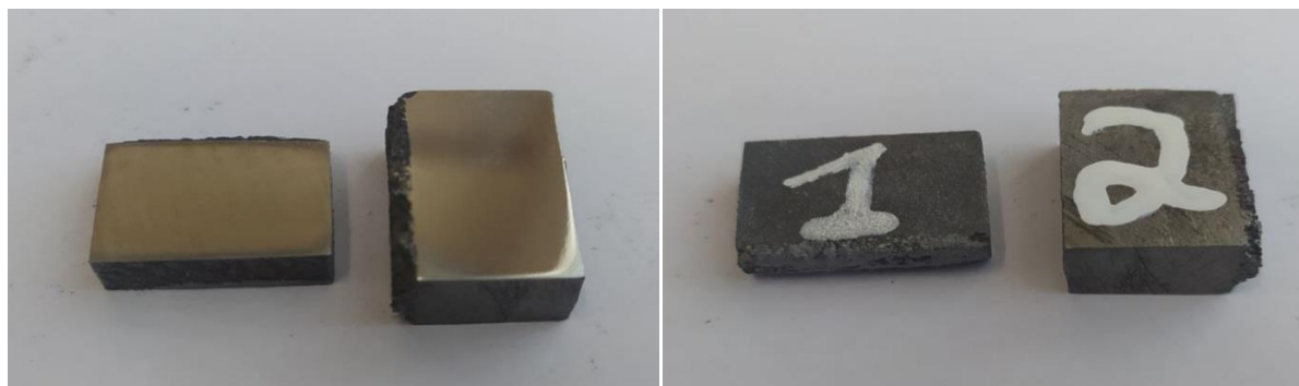
Picture 3. Samples prepared for examination in JSM – IT200 scanning electron microscope.
