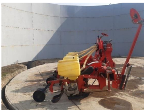
1-rasm. Tuksiz chigitni aniq ekadigan pnevmatik seyalka tajriba nusxasi va traktorga agregatlangan holdagi ko‘rinishi
